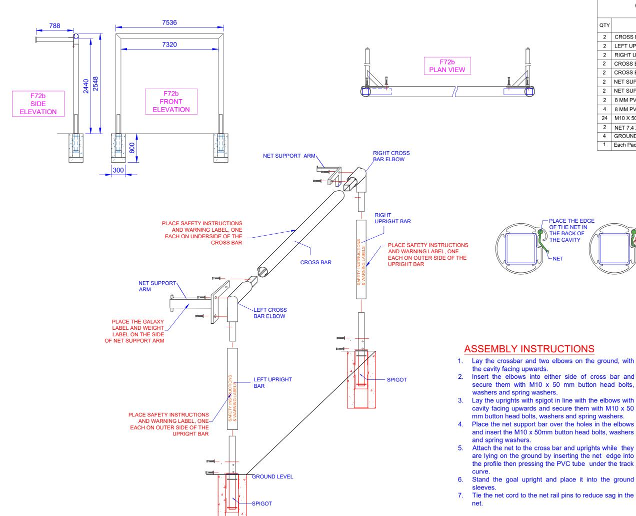
**COMPONENTS** ONE PAIR of GOALS ITEM 2 CROSS BAR 2 LEFT UPRIGHT WITH SPIGOT 2 RIGHT UPRIGHT WITH SPIGOT CROSS BAR ELBOW - LEFT CROSS BAR ELBOW - RIGHT 2 NET SUPPORT BAR - LEFT 2 NET SUPPORT BAR - RIGHT 2 8 MM PVC TUBE 3100 MM LONG 8 MM PVC TUBE 2050 MM LONG 24 M10 X 50 MM S/S HEX HEAD BOLT, WASHER & S/WASHER NET 7.4 X 2.5 X 1.0 X 2.0 M 4 GROUND SLEEVE AND CAP 1 Each Packing, Assembly & Installation sheet
